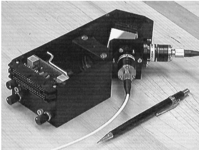
Fig. 12. (a) The optical system layout for the dense-WDM transceiver consists of a 4-f imaging system with the grating placed in the Fourier plane and the OE-VLSI chip placed in the image plane. Pupil-division multiplexing together with a fold mirror is used to separate the modulated wavelength bit-streams into the output fiber. (b) Packaged WDM transceiver.
