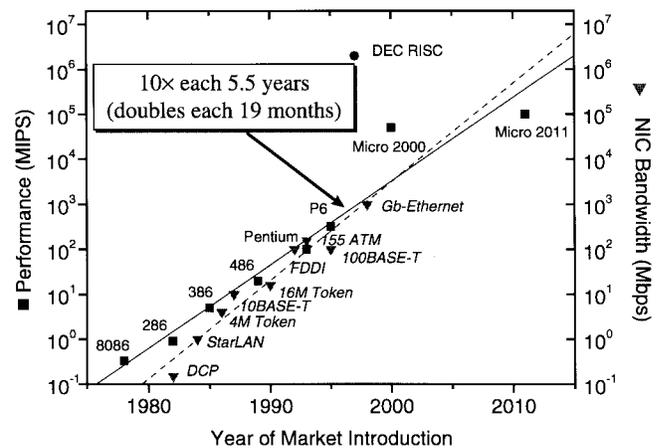
Fig. 1. Evolution of workstation computing performance, measured approximately in millions of instructions-per-second (MIPS), versus network bandwidth, measured in megabits-per-second of the network interface card (NIC).
