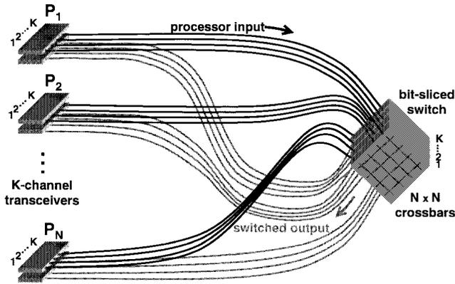
Fig. 3. Architecture of a tightly coupled WDM/SDM multiprocessor network based on the AMOEBIA switch.
