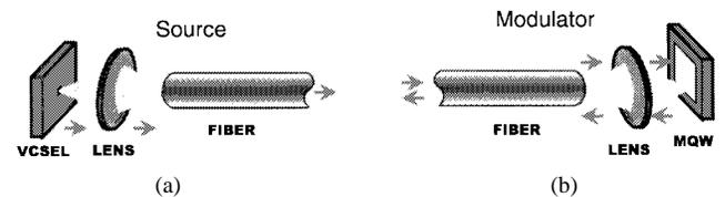
Fig. 8. When coupling an optical source to a fiber (a), the lateral alignment tolerance is determined by the propagating fiber mode. However, when light is coupled out of the fiber and reflected from an oversized modulator back into the source fiber, the lateral alignment tolerance is determined by the modulator aperture.
