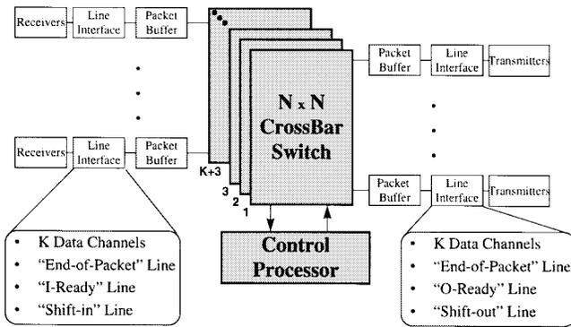
Fig. 2. Architecture of the  $N$ -channel AMOEBA switch. Multiple crossbars (one-per-bit), line interfaces, FIFO-buffers, receivers, transmitters, and controller are incorporated into a single optoelectronic chip.
