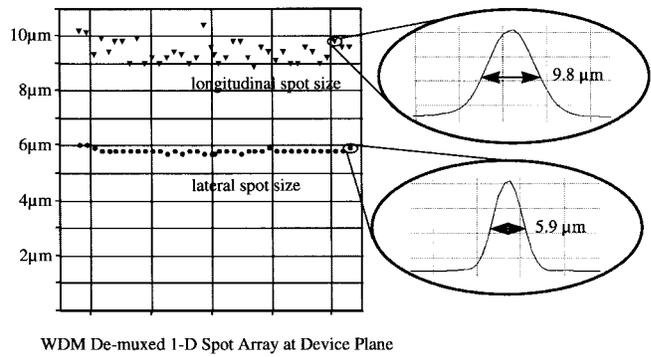
Fig. 13. Performance of the dense-WDM transceiver package. The spot size is relatively independent of wavelength over 38 channels spaced at 0.485 nm ( $35\ \mu\text{m}$  at the chip image plane). The spot position, in addition, is distortion free over a 20 nm range between 843 and 862 nm. Total insertion loss was approximately 10 dB with SMF, and approximately 8 dB with MMF.
