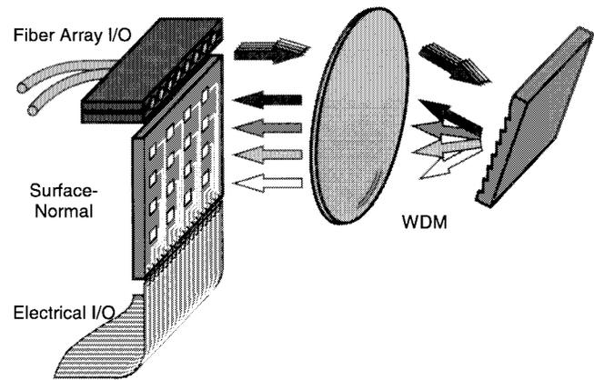
Fig. 7. The combination of space and wavelength division multiplexing enables a 1-D fiber array to access a 2-D array of photonic devices on the optoelectronic switch surface. (Note that the single-fiber transceiver uses a different optical system.)
