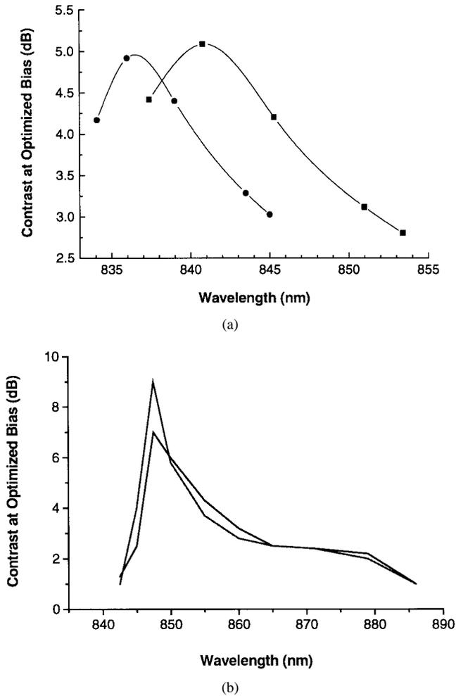
Fig. 19. (a) Predicted performance of a linear MQW modulator array as a function of wavelength, when the voltage swing is constant (4 V), but the bias voltage can be varied across the array. (b) Experimental results from the packaged dense WDM transmitter, verifying that an acceptable contrast ratio (e.g., 2 dB) can be obtained over a wide wavelength range, when multiple bias lines are provided to the array.
