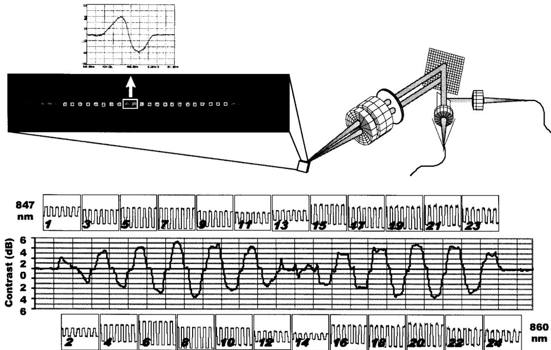
Fig. 18. Experimental results from the 24-channel differential dense-WDM transmitter array when operated in the transmitter package with a fixed bias voltage and a fixed swing of 3 V. Shown are the 24 individual waveforms and the output of an optical spectrum analyzer configured to measure contrast ratio as a function of wavelength.
