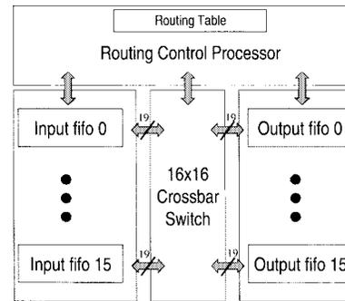
Fig. 4. Block diagram of the AMOEBIA switch.
