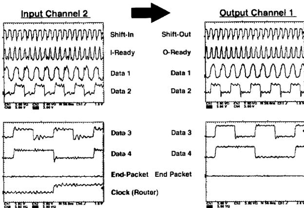
Fig. 6. (a) Measured electrical data from packets flowing through switch from input channel 2 to output channel 1 demonstrating switch operation. Shown are 4 of the 16 data channels at 50 MHz per bit-stream. Shift-in, shift-out, end-of-packet, and the clock to the switch controller (router). (b) Measured optical data from input channel 16 flowing through switch to output channel 16 on the data1 channel.
