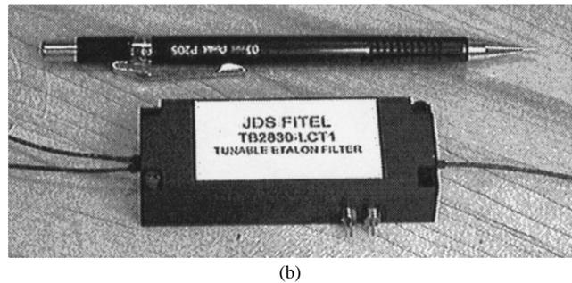
Fig. 14. (a) A tunable etalon filter can be used in this system to provide a narrow, periodic passband for the desired transmission wavelengths. This prevents unwanted light from being imaged onto the chip, and saves power, because the reflected light can again be reused for another transceiver. (b) Picture of the filter fabricated as a custom product by JDS Fitel.
