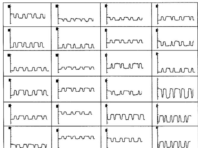
Fig. 17. Optical outputs of a linear column of modulators at 155 Mb/s per bit-stream, configured as a 24-bit dense-WDM transmitter.
