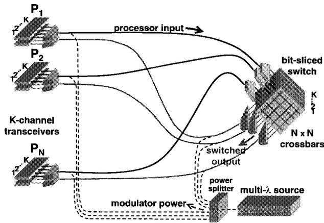
Fig. 11. Fiber-optic WDM/SDM network based on modulators. A short-pulse (100 fs) laser can be used as the broad-band multiwavelength source.
