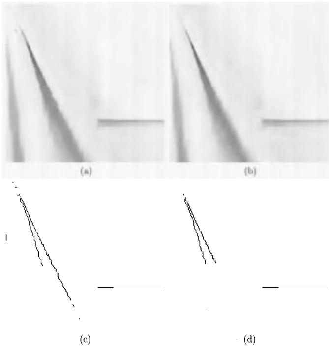
Fig. 9. Staircase effect, a part of the *Bike* image at 0.125 bpp (a) image post-processed by an existing method, (b) image post-processed by the proposed robust filter, (c) edge map of the image processed by an existing method, and (d) edge map of the image processed by the proposed robust filter.
