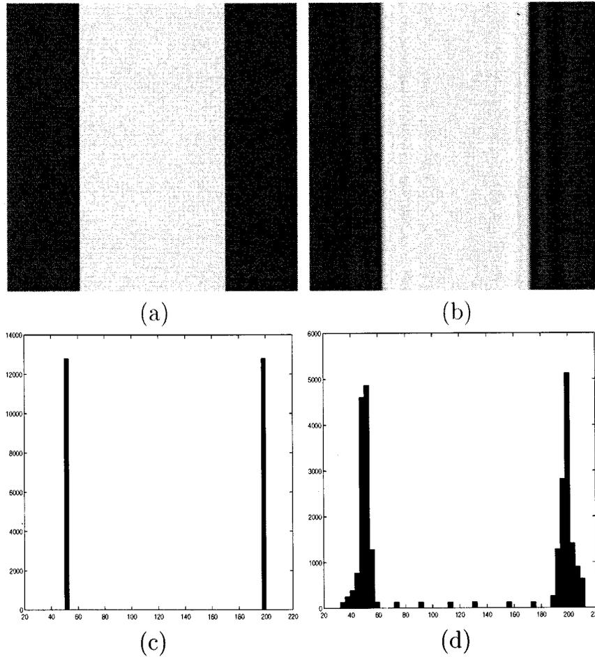
Fig. 1. Degradation by the ringing artifact, an example with a synthetic test images. (a) Original image. (b) Compressed image. (c) Histogram of original image. (d) Histogram of compressed image.
