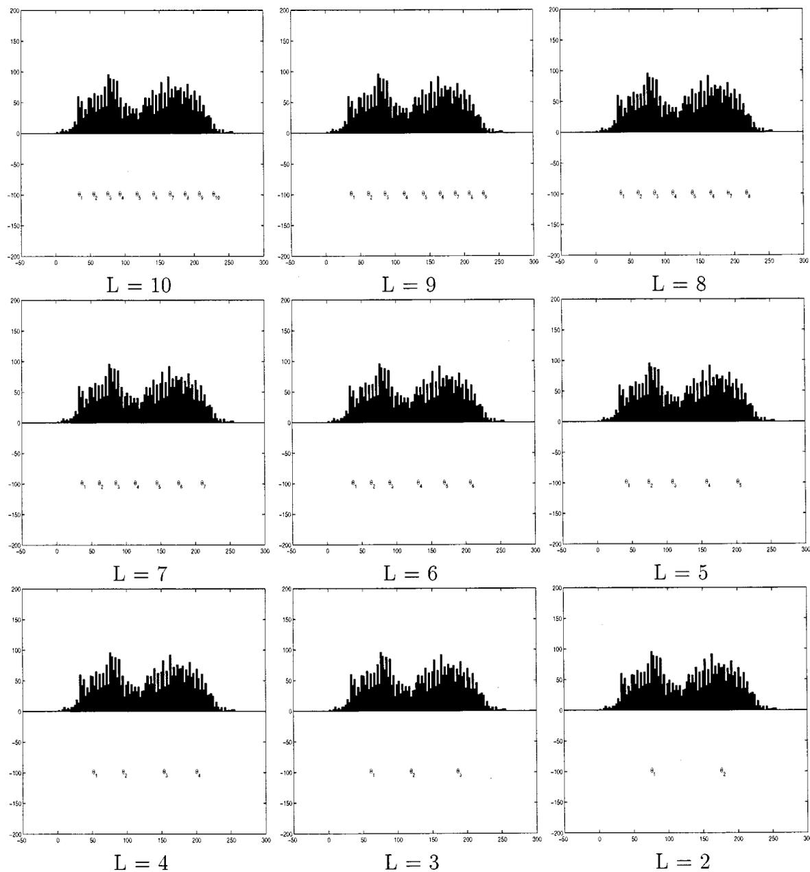
Fig. 4. Example of hierarchical clustering algorithm with the test image (b), cluster center  $\theta$  for  $L = \{2, \dots, K_{\max}\}$  are shown at the bottom of histograms ( $K_{\max} = 10$ ).
