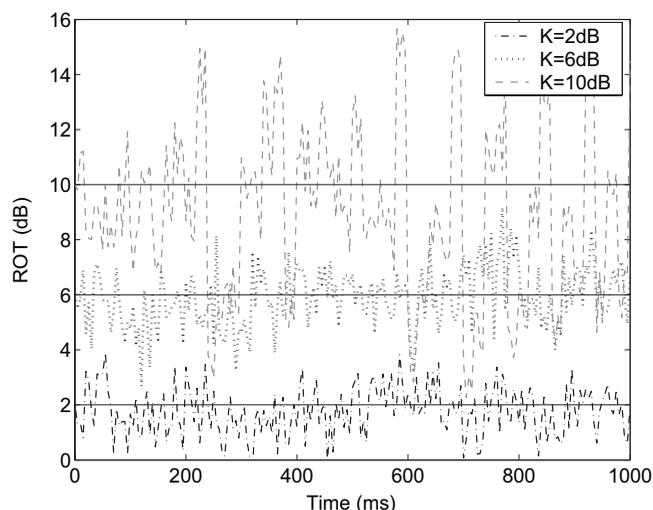
Fig. 7. ROT levels in the presence of dynamic variations for various levels of  $K$  - lower values of  $K$  increase robustness.
