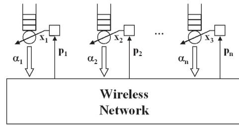
Fig. 1. Distributed feedback structure for rate assignments.
