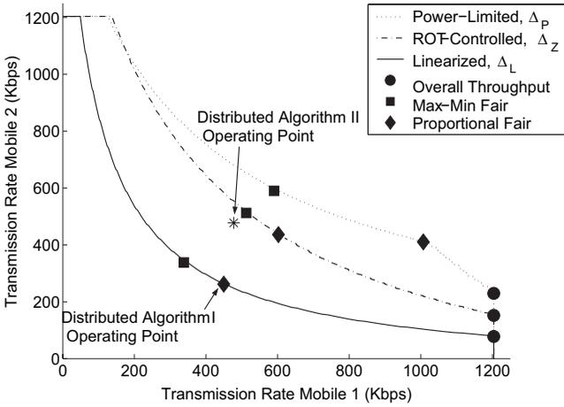
Fig. 2. Power limited, ROT-controlled, and linearized feasibility regions and optimal points of transmission rates.
