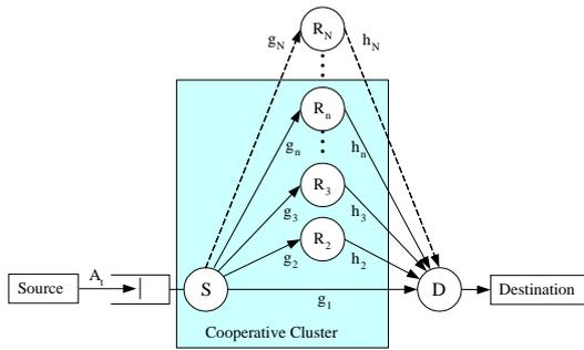
Fig. 1. Cooperative Relay Network with a single bursty source
