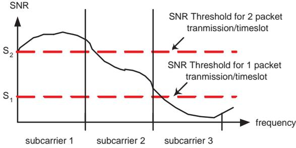
Fig. 1. Mapping of a received SNR channel profile of a user to packet capacity for each subcarrier. In this example, the user can potentially transmit 2, 1, and 0 packets on subcarriers 1, 2, and 3, respectively.
