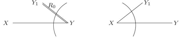
Fig. 4. Cutsets for the primitive relay channel.
