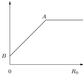
Fig. 6. The achievable rate region for the codebook-aware compress-and-forward coding scheme under a fixed  $p(x)$ .
