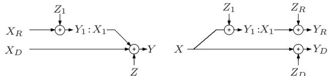
Fig. 2. Gaussian relay channels with orthogonal components.
