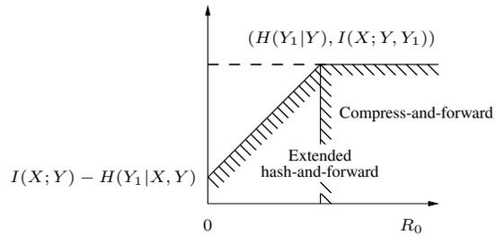
Fig. 5. The comparison of compress-and-forward achievable region (half-open rectangle) and hash-and-forward achievable region (half-open trapezoid) when the relay transfers  $Y_1^n$  faithfully to the receiver.
