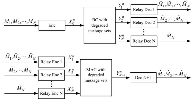
Fig. 3. The modified partial decode-forward scheme.
