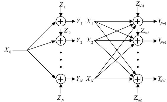
Fig. 1. The Gaussian two-hop relay network.
