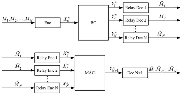
Fig. 2. The partial decode-forward coding scheme by Chern and Özgür.
