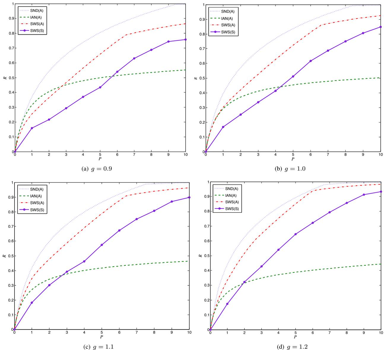
Fig. 4. The transmit power  $P$  vs. achievable symmetric rate  $R$  for the symmetric Gaussian interference channel.
