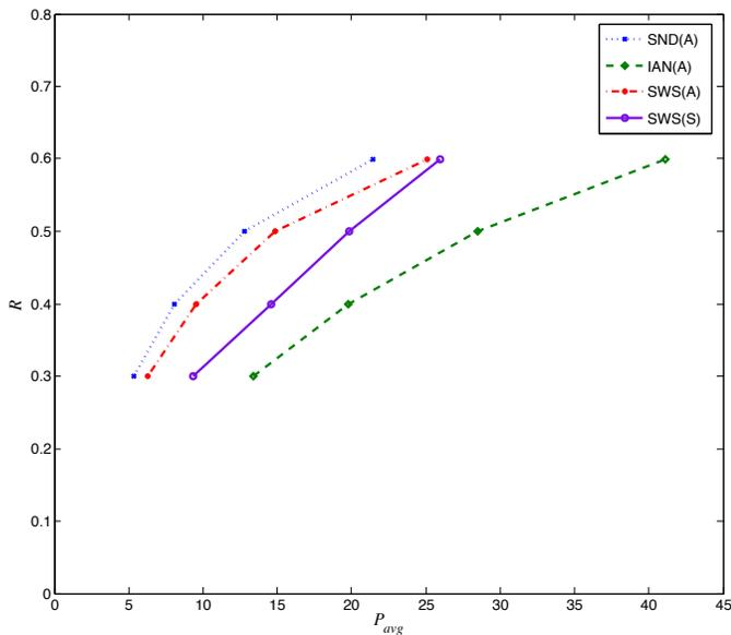
Fig. 5. The average transmit power vs. achievable symmetric rate for the Gaussian interference channel with random coefficients.
