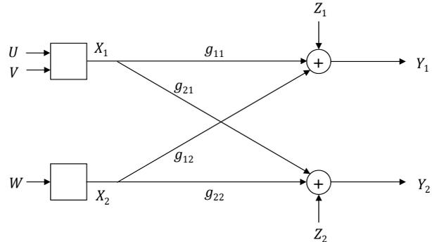
Fig. 2. Superposition coding with virtual input signals  $U$ ,  $V$ , and  $W$ .
