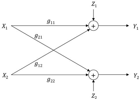
Fig. 1. The two-user Gaussian interference channel.
