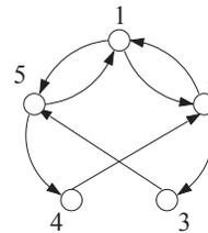
Fig. 4. An index coding problem with  $\beta = 3 < b(\mathcal{R}_{LTS}(G)) = b_{LTS}(G) = 7/2$ . Here  $\beta$  is achieved by composite coding [14].
