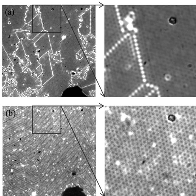
FIG. 3. Images of the dual-layer polystyrene bead lattice (diameter  $\sim 2 \mu\text{m}$ ), obtained using (a) the conventional DF microscopy and (b) the plasmonic DF microscopy. The top layer of the beads is clearly imaged by the conventional DF microscopy and shown as white in-line dots in (a). The PDF microscopy clearly resolves the bottom layer of the beads, as shown in (b). Note that the bright areas in (b) are artifacts.
