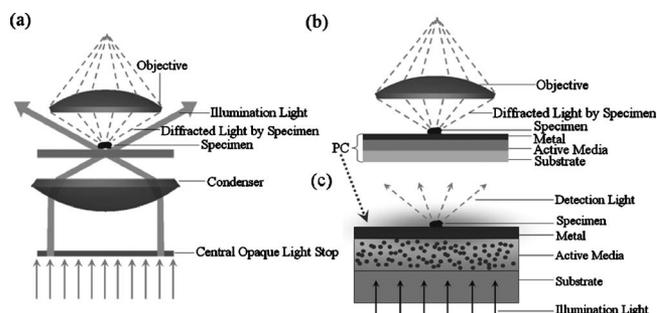
FIG. 1. Schematic configurations of (a) conventional DF microscopy, (b) plasmonic DF microscopy and (c) PC.
