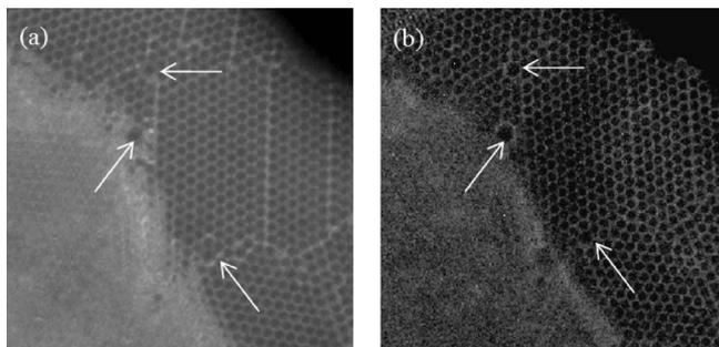
FIG. 2. Images of the monolayer polystyrene bead lattice, obtained using (a) the conventional DF microscopy and (b) the plasmonic DF microscopy. The lattice is composed of self-assembled monolayer of polystyrene beads (diameter  $\sim 2 \mu\text{m}$ ).
