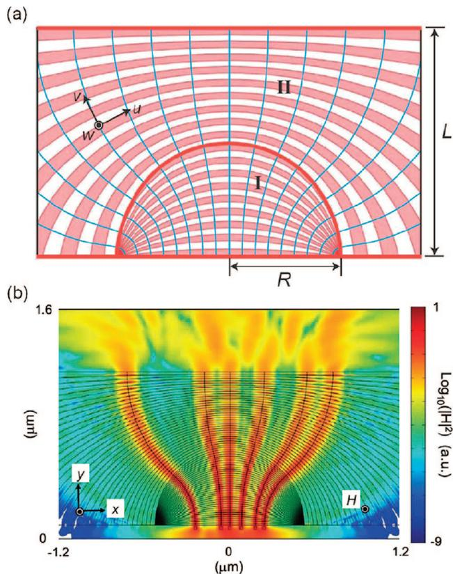
**Figure 3.** New metamaterial-based optical element: *optical transformer*. (a) Scheme of the optical transformer consisting of two domains of alternating curved layers of Ag (pink) and GaN (white). The light flows along the  $v$  axis (curved blue lines), and the interfaces between the layers comply with the  $u$  axis. (b) Magnetic field intensity profile showing subwavelength imaging and magnification of the optical transformer.
